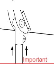
Ensure shaft is fully inserted into neck assembly.
